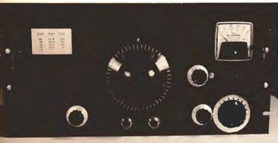
FRONT PANEL VIEW of the hetrodyne exciter. Pilot lamps have since been moved to left side of panel to make room for "zero-in" push-button switch and signal level control below tuning dial. Another good quality type of dial also can be used on the exciter, if available, such as the Eddystone type 898 dial.
