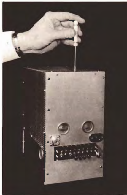
REAR VIEW of the amplifier. Locations for J 1 , J 2 , the high voltage connector, and terminal strip TS 1 can be determined from this view. Note ventilating snap-in buttons on sides and back.
