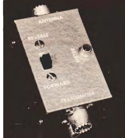
TOP VIEW of the RF pickup unit. Compact size and complete shielding contribute to maintaining 50-ohm impedance through unit, minimizing disturbance in line. Box size is 3¼ x 2½ x 1⅞ inches.
