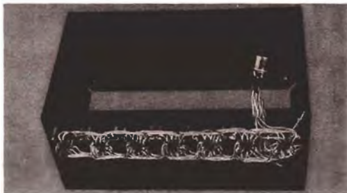
FIG. 2. ACCESSORY SOCKETS were first fastened to the outside of the cabinet bottom, wired and then mounted inside the box. Cut metal spacers to length that allows lugs on sockets to clear metal box.
