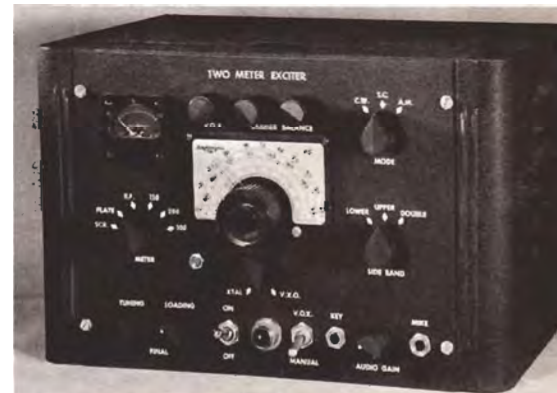
FRONT-PANEL VIEW of the complete exciter constructed in an 8x12½x8-inch steel cabinet. All controls used during normal operation are on the front panel. The National MCN dial tunes the VXO over 100-kilocycle segments.
