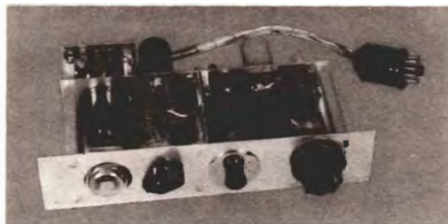
FIG. 1. SIDE VIEW of the COMBO MONITOR unit. Corner posts connecting the panel and chassis are 3 inches long. Those for the 2 x 2¼-inch mounting plate for the 1-megohm potentiometer are 1½ inches long. All posts are tapped for 6-32 screws at both ends.
