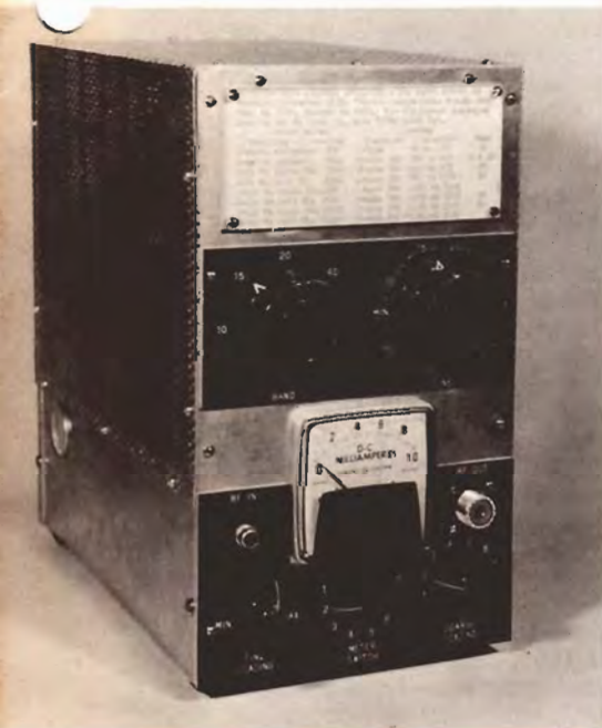
CLOSEUP FRONT VIEW of the SSB-600 amplifier. Note complete operating instructions at top of panel (see copy on page 7). Markings for panel controls were engraved on black plastic name plate material.
