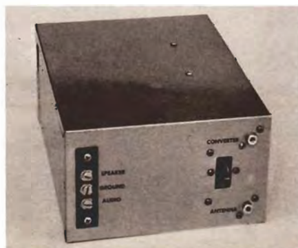
REAR VIEW of the receiver, showing the positions of the antenna and output jacks, power plug and audio terminal strip.
