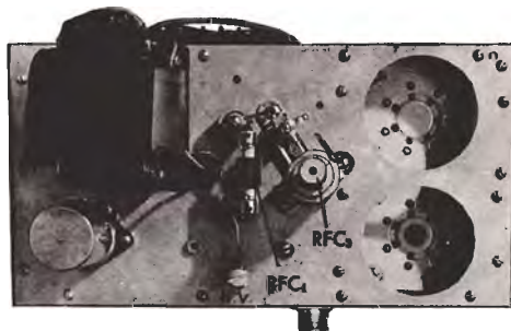
RIGHT REAR VIEW of the linear amplifier. Note how C_1 and C_2 are mounted on vertical brackets made from \frac{1}{8} -inch thick sheet aluminum. The copper angle brackets and U-shaped angle bracket on C_1 is S_2 (See FIG. 5 for details). A 6 x 11 x 2 \frac{1}{2} -inch aluminum chassis houses most of the smaller components in the amplifier.
