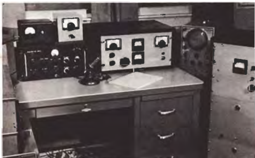
MONITOR-ADAPTED 'SCOPE AT K21OW, at right of desk, a Heath type O-5 constructed from a kit. Space for the adapter components and additional panel controls can be found in most test type oscilloscopes.
